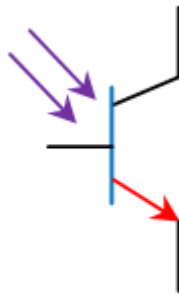
Figure: Symbol for photo transistor
